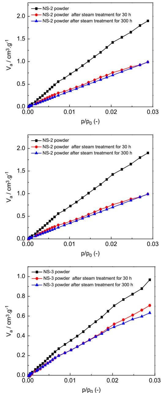
Fig. 11.  $CO_2$  adsorption isotherms (at 298 K) for the 450 °C-calcined NS powders before and after hydrothermal treatment (powders were hydrothermally-treated in an autoclave at 180 °C for 300 h).
