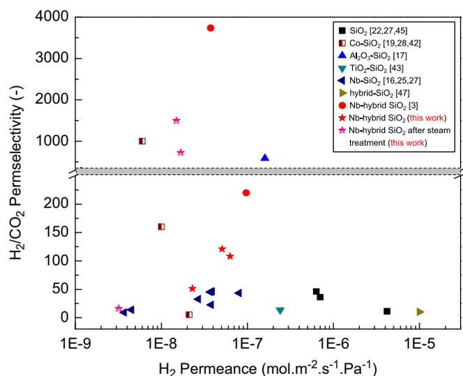
Fig. 1. Comparison of performances of NS membranes (this work) with that of microporous silica and modified silica-based membranes in terms of  $\text{H}_2$  permeance and  $\text{H}_2/\text{CO}_2$  permselectivity.
