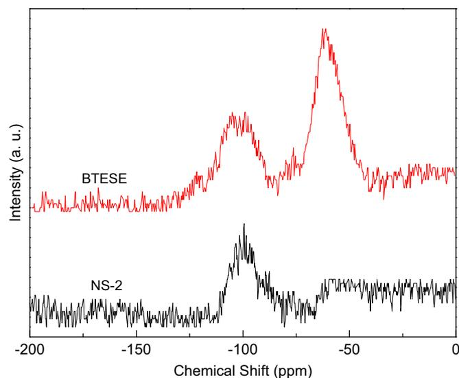
Fig. 7.  $^{29}\text{Si}$  MAS NMR spectra of the BTESE and NS-2 powders.
