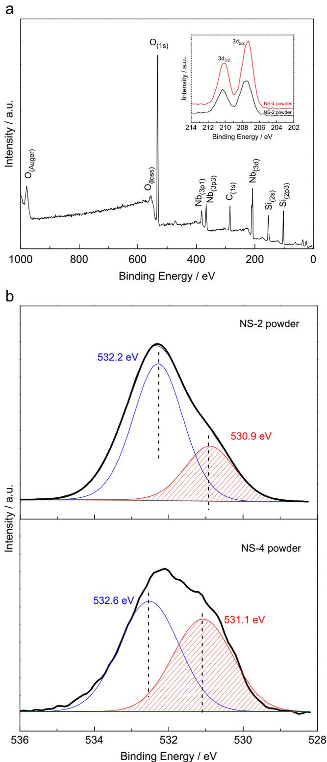
Fig. 6. (a) XPS spectrum of NS powder. Also shown inset is the spectrum of the Nb 3d<sub>5/2</sub> and Nb 3d<sub>3/2</sub> regions for NS-2 and NS-4 powders. (b) XPS spectrum of the O 1s region for NS-2 and NS-4 powders, which is fitted with a Gaussian distribution.
