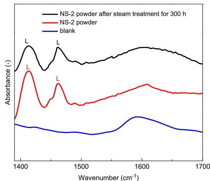
Fig. 4. Py-IR spectra of NS-2 powder before and after steam treatment (1000 kPa for 300 h) that measured at  $200^\circ C$ .
