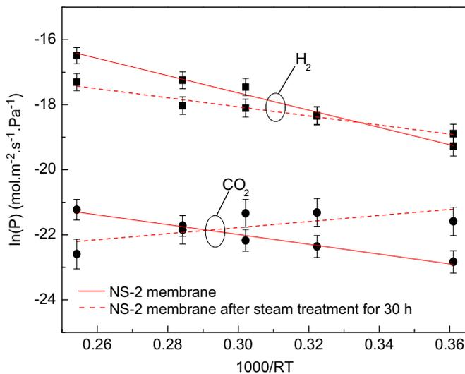
Fig. 10. Arrhenius plot of the  $H_2$  and  $CO_2$  permeance through NS-2 membrane before and after steam treatment for 30 h.
