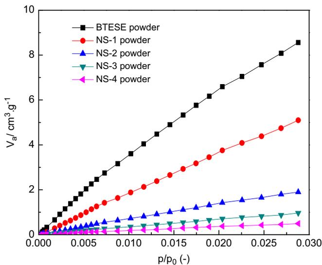
Fig. 5. CO<sub>2</sub> adsorption isotherms (at 298 K) for the calcined BTESE and NS powders.
