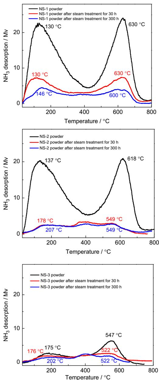
Fig. 12. NH<sub>3</sub>-TPD spectra of the calcined NS powders before and after steam treatment.
