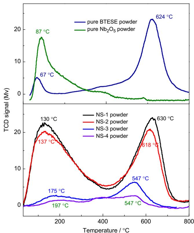
Fig. 3.  $NH_3$ -TPD curves of hybrid  $SiO_2$ (BTESE),  $Nb_2O_5$  and NS powders.
