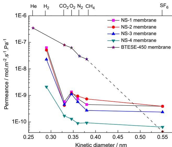
Fig. 2. Single gas permeances of 450 °C-calcined BTESE and NS membranes as a function of the kinetic diameter of the permeating gas molecule measured at 200 °C and 0.3 MPa.
