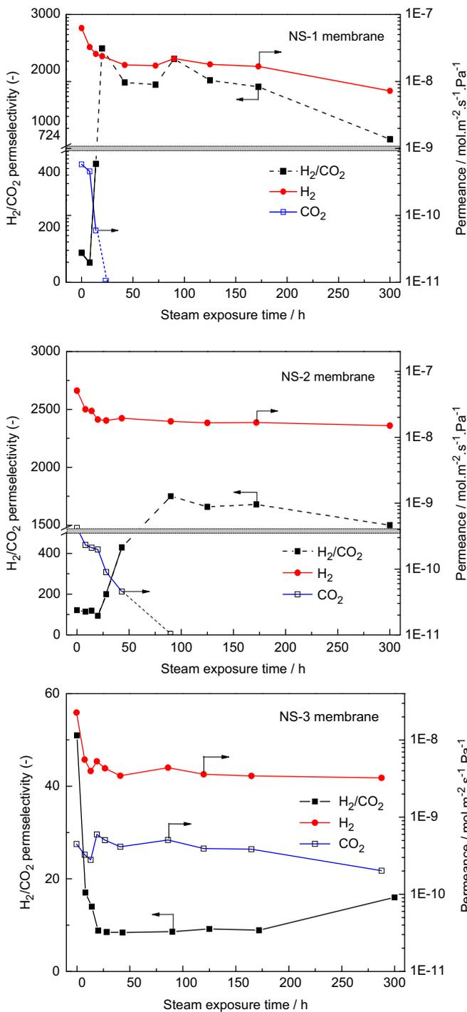
**Fig. 9.** Hydrothermal stability test of NS-1, NS-2 and NS-3 membranes. (Shown are the H<sub>2</sub> and CO<sub>2</sub> gas permeances at 200 °C and the calculated single gas H<sub>2</sub>/CO<sub>2</sub> selectivity as a function of the time of exposure to 150 kPa steam).
