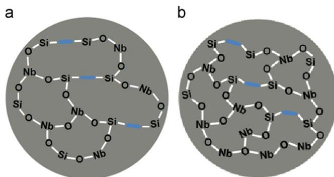
Fig. 8. Schematic representation of Nb-hybrid  $\text{SiO}_2$  networks (a) Nb-hybrid  $\text{SiO}_2$  with low Nb content, (b) Nb-hybrid  $\text{SiO}_2$  with relatively high Nb content.
