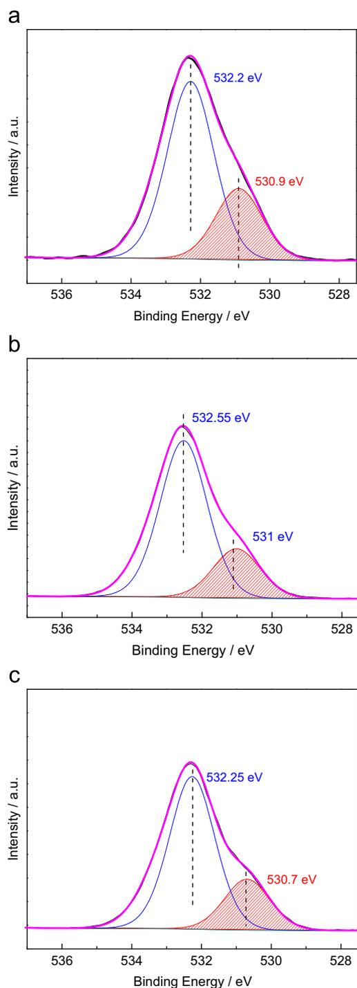
**Fig. 13.** XPS spectrum of the O 1s region for the calcined NS powders before and after hydrothermal treatment, which is fitted with a Gaussian distribution. (a) NS-2 powder. (b) NS-2 powder after hydrothermal treatment for 30 h. (c) NS-2 powder after hydrothermal treatment for 300 h.
